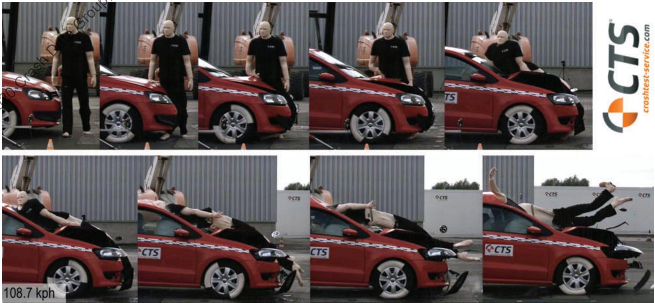
**Figure 3: Motion sequence of the Biofidel dummy at  $v = 109$  kph.**
