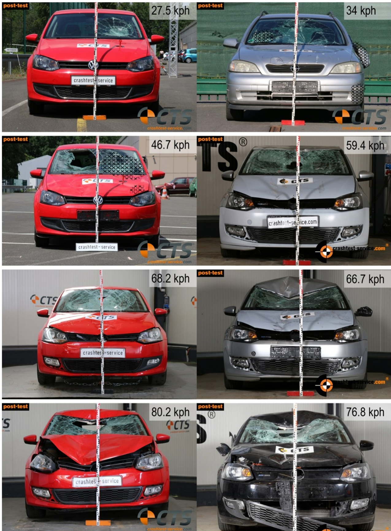
Figure 5 : Comparison of the damage to the VW Polo 6R after an impact with the biofidelic dummy (left) and a conventional dummy (right) with increasing collision velocity (frontal view)
