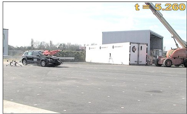
Figure 2. : Re-enactment (left – biofidelic) of the already available crash tests (right – conventional). Collision velocity here: v = 68 kph
