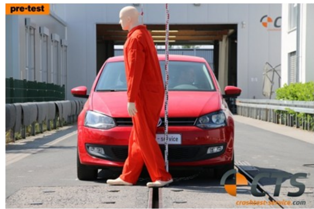
Figure 1. : Crash test vehicle VW Polo 6R (left) and impact configuration with a biofidelic dummy (right) for the crash series performed
