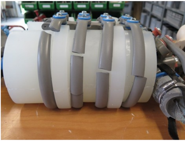
Figure 12 : Biofidelic dummy with serial rib fracture and shoulder joint injuries at a collision velocity of approx. 70kph
