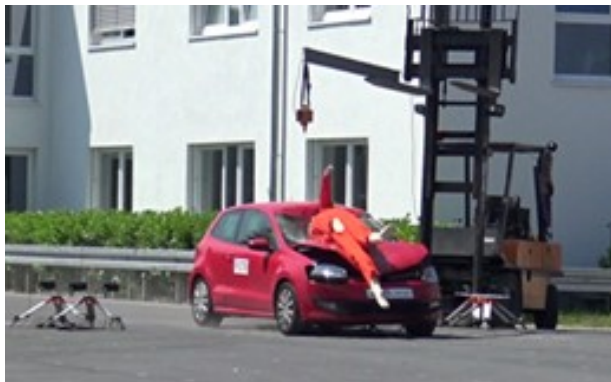
Figure 2. : Re-enactment (left – biofidelic) of the already available crash tests (right – conventional). Collision velocity here: v = 68 kph
