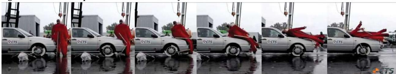
**Figure 5: Movement sequence of the biofidelic dummy in crash test (mirrored)**
