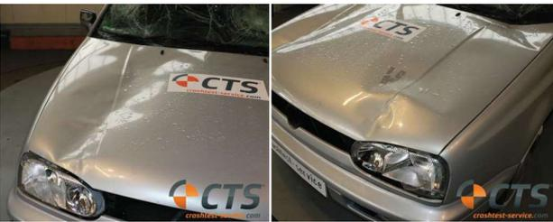
Figure 8: Kontakt marks on the bonnet from the NAMI (L) and the biofidelic dummy (R)
