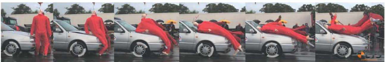
**Figure 4: Movement sequence of the NAMI-dummy in crash test**
