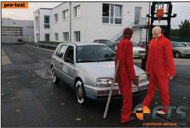
**Figure 3: Impact configuration: conventional dummy left, biofidelic dummy right**
