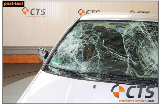
Figure 7: Fracture pattern on the windshield
