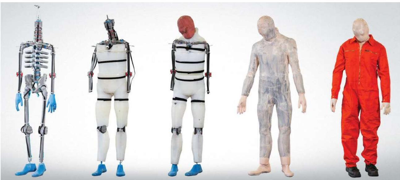
**Figure 2: Production stages of a Biofidelic Dummy**
