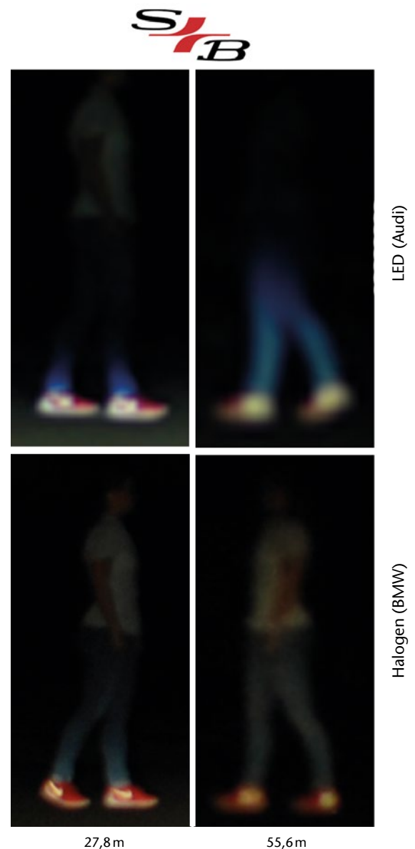
FIGURE 15: View from a distance of 27.8 and 55.6 m with LED (Audi) and halogen (BMW)
