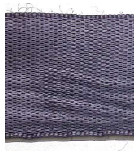
BILD 10: Gurtband Sicherheitsgurt Lkw-Gurtschlittens nach zirka 3000 Versuchen FIGURE 10: Seat belt strap of a truck seat belt testing sled after approximately 3,000 tests
